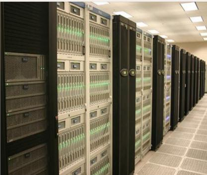
The Ranger system is comprised of 3,936 16-way SMP compute nodes providing 15,744 AMD Opteron
